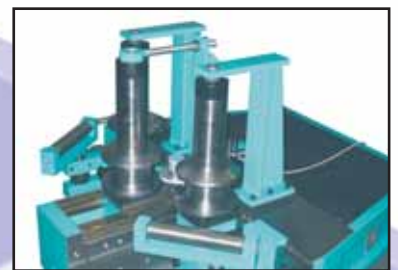
Special design with 400 mm shaft length and shaft support
