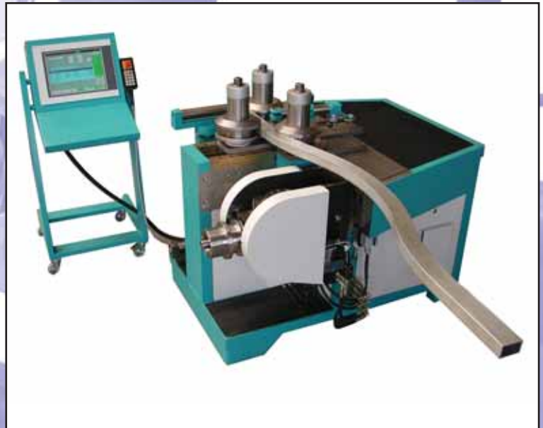
RB3 with universal axis swivelled down (vertical direction)
