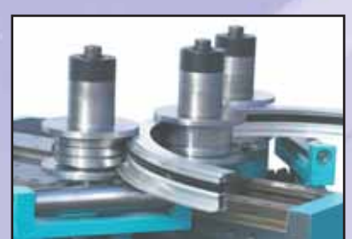
RB3 with special rolls for frame sections
