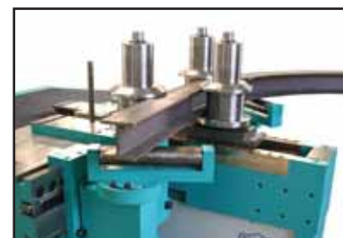
RB4 with steel section
